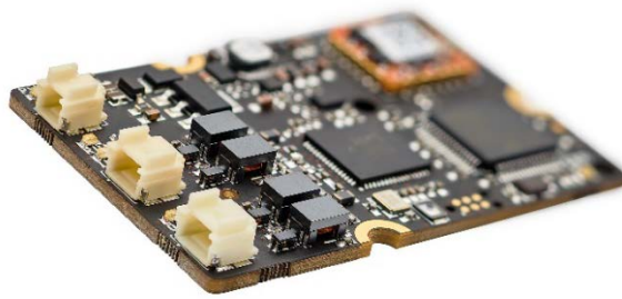
Figure 3: Connectors on front side (PCB-version)
