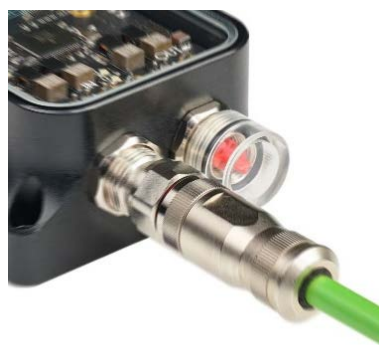
Figure 15: Screw Cap Mounting for IP67 rating
