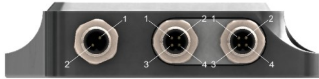
Figure 5: Connector pin locations HSD-version
